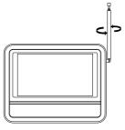
Hold the direct-connect antenna and rotate the nut as shown below to remove.
